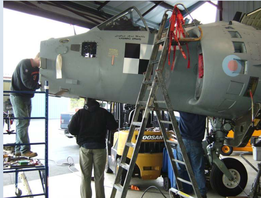
Once the airplane was on jacks, we were able to disassemble the nose and begin our detailed inspections. The reaction controls, nose landing gear doors and all panels were removed.
